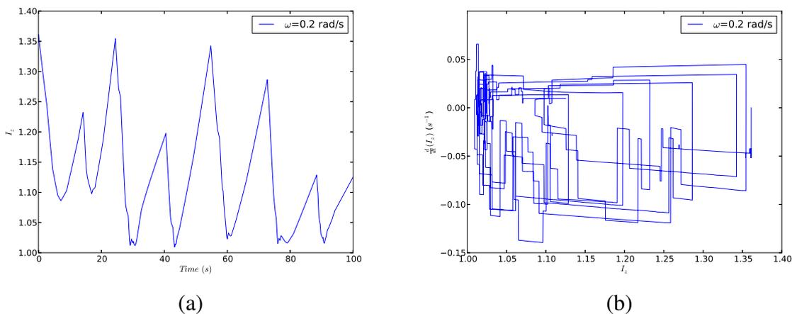
Figure 4: (a) Mass inertia index time evolution  $I_z$  and (b) phase plane diagram of the mass inertia index of the stack with initial gap  $g = 6$  mm for constant velocity amplitude  $A = 2.4$  mm/s and excitation frequency  $\omega = 0.2$  rad/s.
