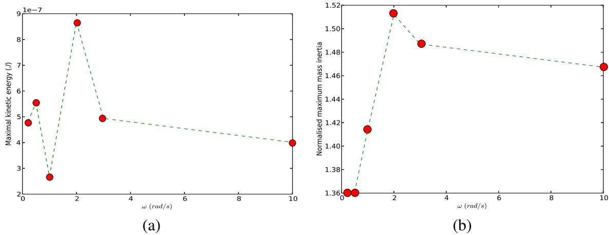
Figure 3: (a) Maximum relative kinetic energy and (b) maximum mass inertia achieved by the block system according to excitation frequency  $\omega$  with initial gap between blocks  $g = 6$  mm for velocity amplitude  $A = 2.4$  mm/s.
