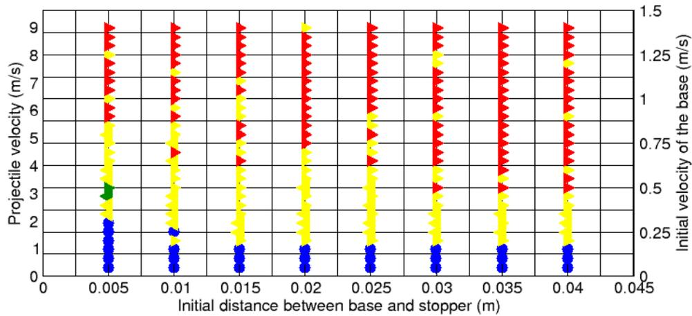
Figure 13: Modes of overturning from computational simulations of the dynamic behaviour of a stack of three blocks (*Scale 1*) due to pulse-type excitation
