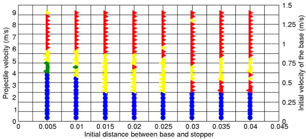
Figure 15: Modes of overturning from computational simulations of the dynamic behaviour of a stack of three blocks (*Scale 2*) due to pulse-type excitation
