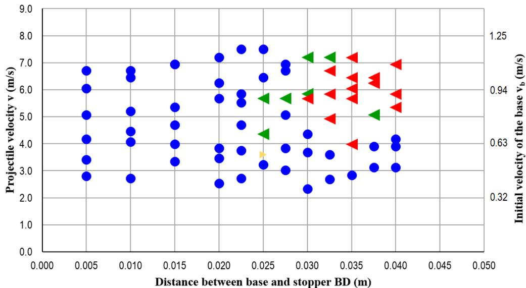
Figure 12: Modes of overturning from experiments with a stack of three blocks (*Scale 1*) due to pulse-type excitation
