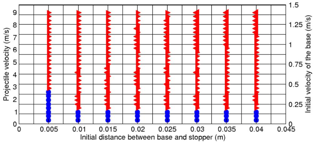
Figure 7: Modes of overturning from computational simulations of the dynamic behaviour of a single block (*Scale 1*) due to pulse-type excitation
