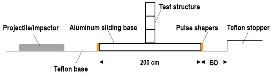
Figure 1: Experimental set-up scheme at Impact Engineering Laboratory in Oxford
