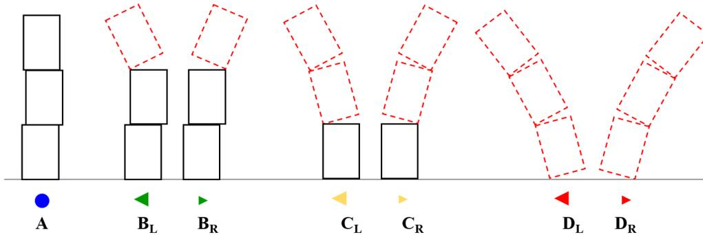
Figure 11: Modes of overturning of stack of three blocks
