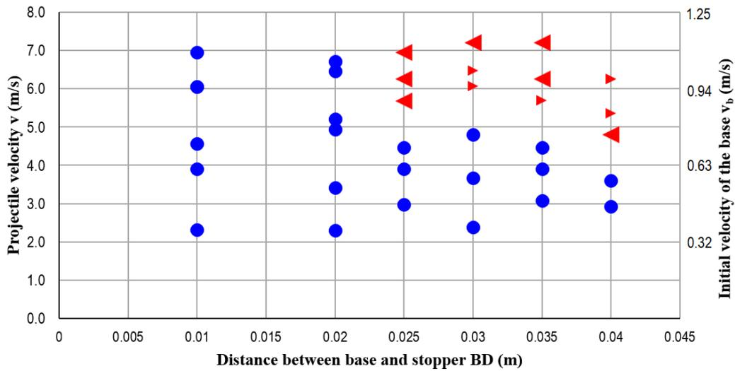
Figure 8: Modes of overturning from experiments with a single block (*Scale 2*) due to pulse-type excitation
