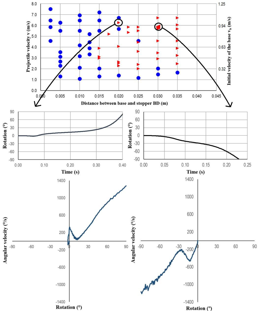
Figure 17: Rotation histories and phase-plane views of rotations from two experiments with a single block (*Scale 1*) and initial conditions  $BD$  2 cm and  $v = 6.25 \frac{m}{s}$  (graphs on the left side) and  $BD$  3 cm and  $v = 5.86 \frac{m}{s}$  (graphs on the right side)
