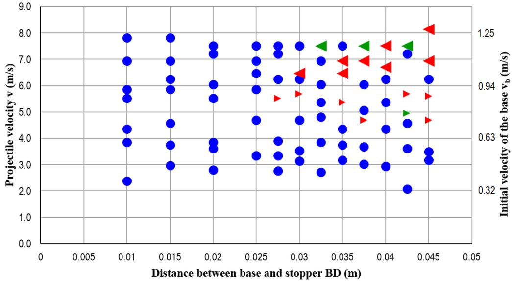
Figure 14: Modes of overturning from experiments with a stack of three blocks (*Scale 2*) due to pulse-type excitation
