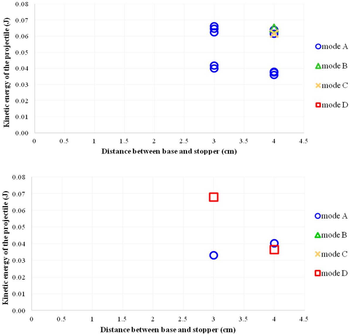
Figure 7: Modes of failure for stack of three blocks with smooth (above) and non smooth (below) contacts related to kinetic energy of the projectile and the distance between the aluminium base and the stopper
