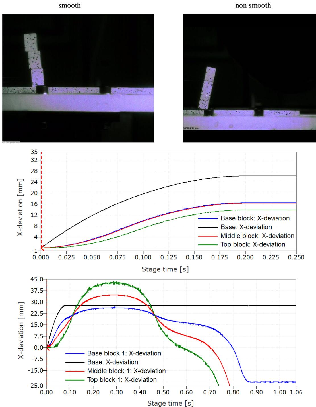
Figure 6: Typical horizontal displacement histories for the base and blocks centroids, for the case of smooth (above) and non smooth (below) contact surfaces
