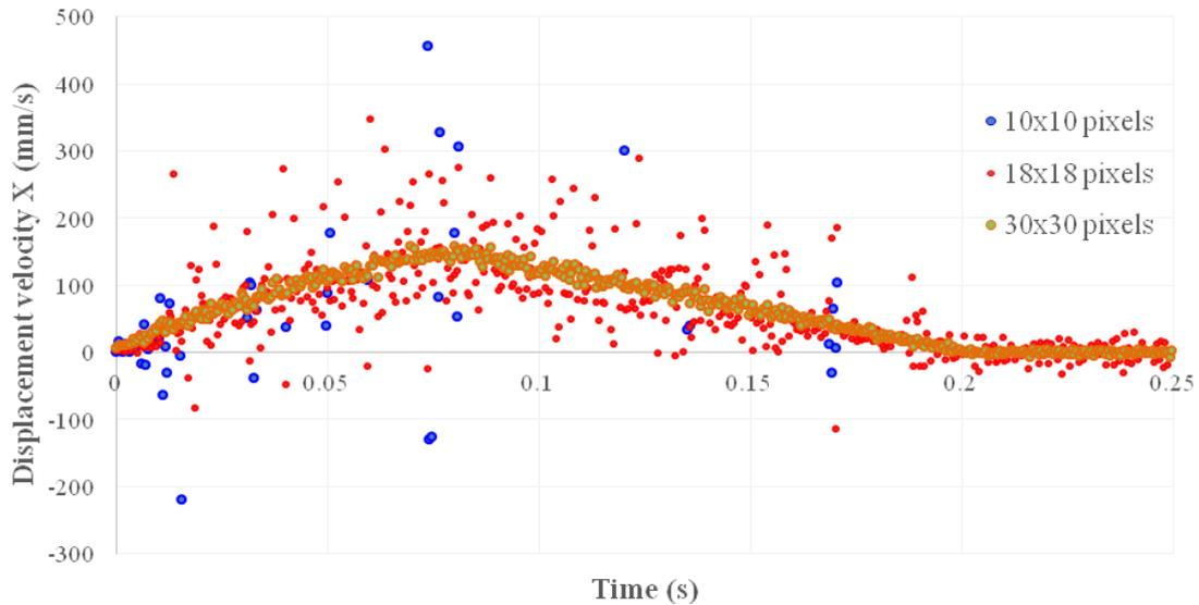
Figure 4: Velocity of the bottom block for a three blocks stack using different Aramis facet resolutions
