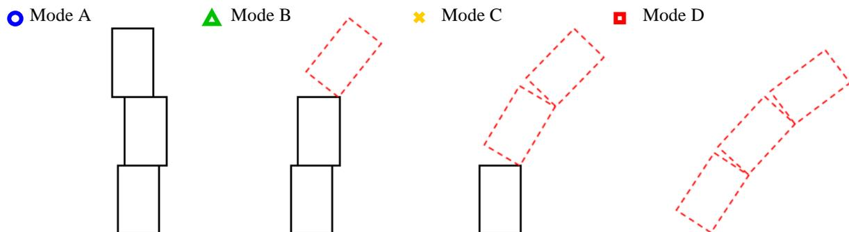
Figure 5: Possible modes of failure of the stack of three blocks
