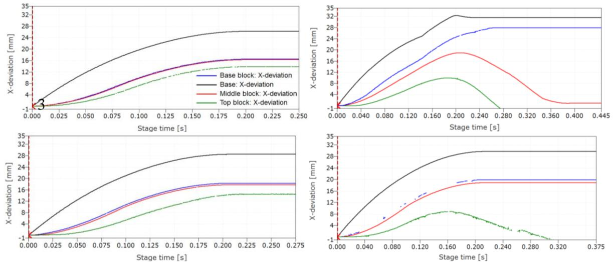
Figure 3: Displacement of base, bottom, middle and top block from four repetitions of experiment B3\_IM10\_BD4 (3 blocks, spring trigger position 10, distance to stopper 4 cm) – smooth contact surfaces
