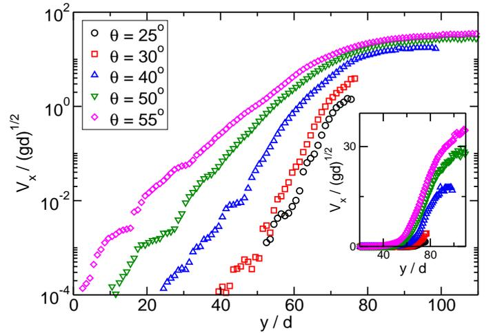
Figure 3: (Color online) Semi-log velocity profiles  $V_x/\sqrt{gd}$  at inclinations shown versus depth  $y/d$  (inset: linear-linear profiles) for friction coefficient  $\mu_g = 0.3$  and  $\mu_w = 0.3$ .
