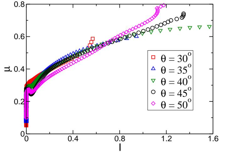
Figure 5: (Color online) The effective coefficient of friction  $\mu = \tau/P$  at inclinations shown versus inertial number  $I$  for friction coefficients  $\mu_g = 0.3$  and  $\mu_w = 0.6$ .
