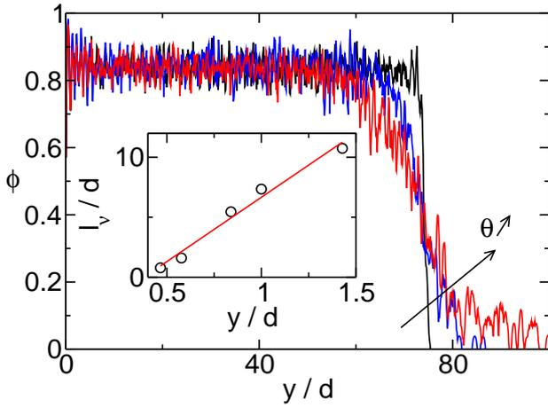
Figure 2: (Color online) Vertical profile of solid fraction  $\phi$  at inclinations shown versus depth  $y/d$  (the bottom of the cell is located at 0) for  $\mu_w = 0.3$  and  $\mu = 0.3$ . Inset variations of the scale  $l_\nu$  with  $\tan \theta$ . The dashed line corresponds to the best fit.
