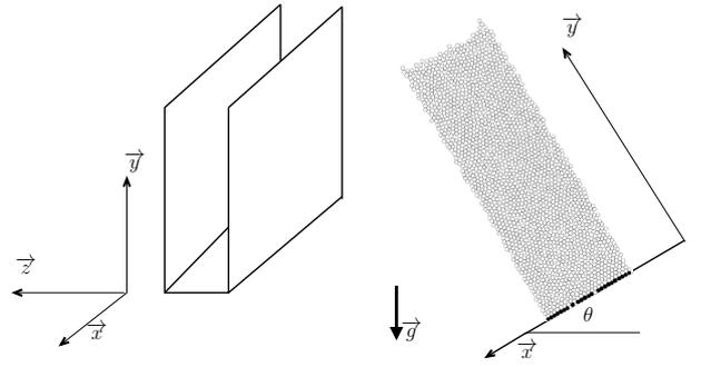
Figure 1: Sketch of the set-up and cartesian coordinate system with unit vector  $\mathbf{x}$  along the flow, normal to the free surface and perpendicular to sidewalls with origin at the bottom of the cell.
