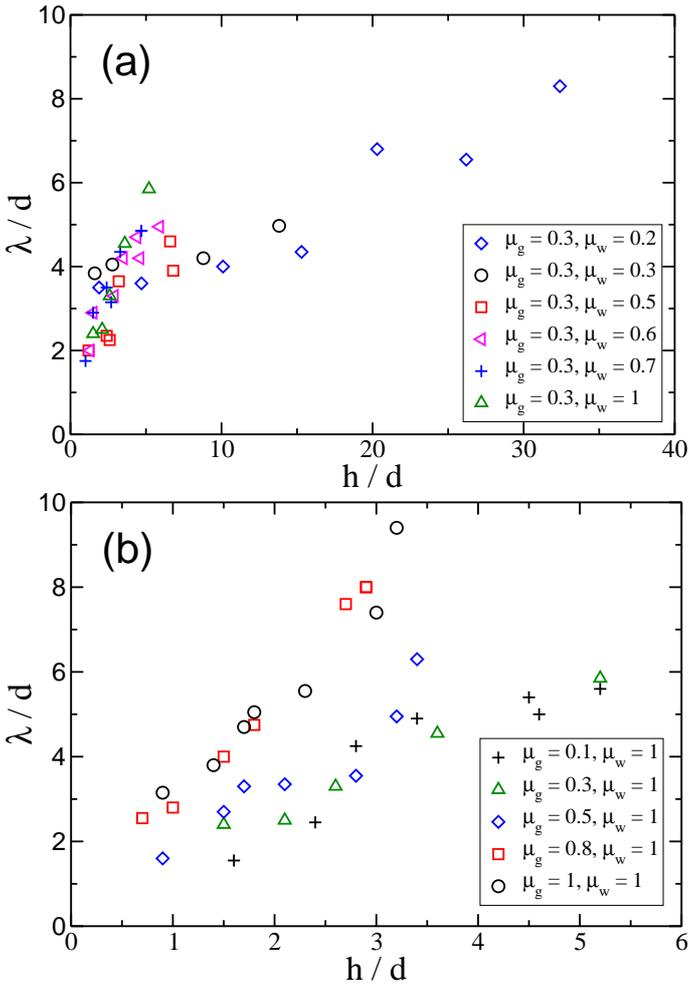
Figure 4: (Color online) Characteristic length of the velocity decay  $\lambda$  versus the height  $h$  of the flowing zone with (a) constant friction coefficient  $\mu_g = 0.3$  and (b) constant friction coefficient  $\mu_w = 1$ .
